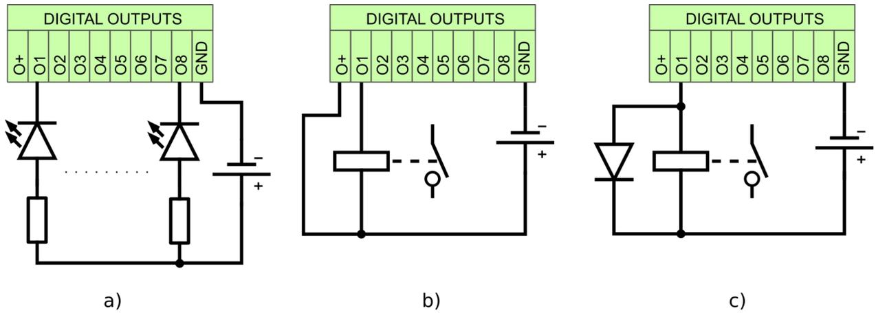
Fig. 3. Example digital outputs connections: (a) LED, (b,c) relay
