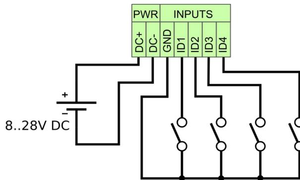
Fig. 1. Power supply and dry contact inputs connections
